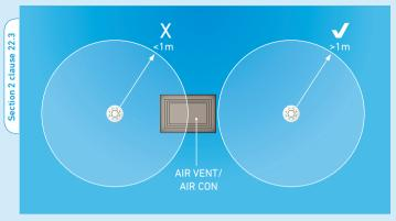
Do not site detectors less than 1m from air supply points or air circulating units.
