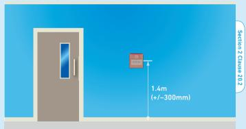
The centre of the element of the manual call point should be positioned 1.4m (+/-300mm) from floor level. Unless a wheelchair user is likely to be the first person to raise the alarm. (Between 800-1200mm according to Doc. M. + Equality Act). BS 5839 states transparent hinged covers should be fitted to all manual call points.
