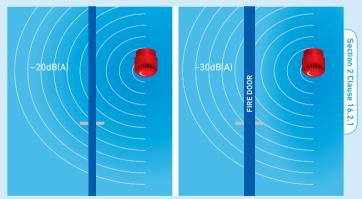
Decibel loss occurs through doors: approximately –20dB(A) through a normal door, and approximately –30dB(A) through a fire door. Unless a sounder is installed in a bedroom, it is unlikely that 75dB(A) will be achieved.
