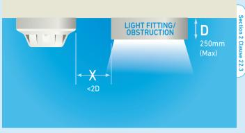
Never mount devices closer than twice the depth of light fittings or other obstructions on the ceiling.
