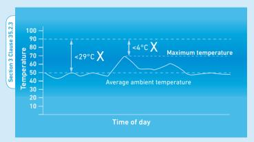
The minimum static response to heat devices should not be less than  $29^{\circ}$ C above the average ambient temperature, or less than  $4^{\circ}$ C above the highest temperature the device can expect to experience.
