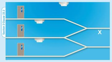
Enclosed stairways should have a detector at the top of the stairway and on each main landing.
