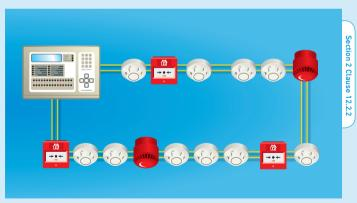
Short circuit isolators limit the effect of one fault to 2000m<sup>2</sup> and to a single storey of the building. '2 simultaneous faults on a circuit should not disable protection within an area greater than 10,000m<sup>2</sup>.
