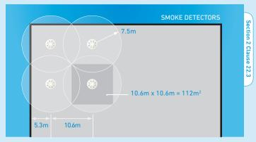
When mounted on a flat ceiling, smoke detection devices have an individual coverage of 7.5m radius. However these radii must overlap to ensure there are no 'blind spots'. Therefore individual coverage can be represented by a square measuring 10.6m x 10.6m giving an actual area coverage of 112m<sup>2</sup> per device.
