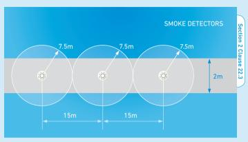
In corridors less than 2m wide the horizontal spacing of detectors may be increased, the areas of coverage need not overlap as in the case of a room. Any corridor over 2m wide is deemed a room and device spacing should follow the standard for rooms (see page 9).
