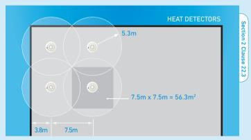
When mounted on a flat ceiling, heat detection devices have an individual coverage of 5.3m radius. However these radii must overlap to ensure there are no 'blind spots'. Therefore individual coverage can be represented by a square measuring 7.5m x 7.5m giving an actual area coverage of 56.3m<sup>2</sup> per device.
