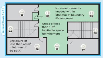
The minimum sound level should be 65dB(A) or 5dB(A) above a background noise which is louder than 6ddB(A) (if lasting more than 30 seconds) and at a frequency of between 500Hz and 1000Hz. The maximum sound level should not be greater than 120dB(A) at any normally accessible point. May be reduced to 60dB(A) in stairways, enclosures up to  $60m^2$  and specific points of limited extent.
