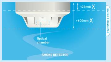
The sensing element of a smoke detection device (optical smoke or ionisation chamber) should not be less than 25mm below ceiling, and not greater than 600mm below ceiling.
