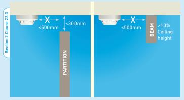
A device should not be mounted within 500mm of any obstruction.
